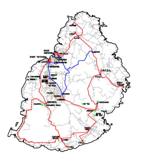
The transmission network, operates at 66 kV, transporting power in bulk from the main sources of generation to **eighteen** 66kV-22kV substations scattered over the island.
