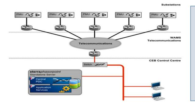
Current, voltage and frequency measurements are taken by the PMU and stored in a data concentrator. The measured quantities include both magnitudes and phase angles, and are time-synchronised via Global Positioning System (GPS) receivers with an accuracy in microsecond.
