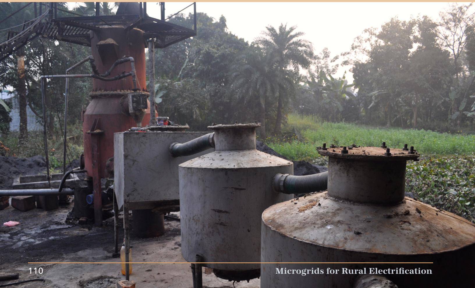
A Husk Power Systems biomass gasifier in Bihar, India.
