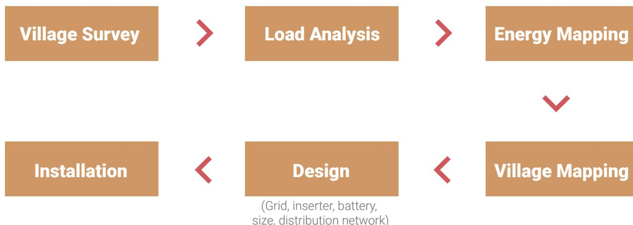
Table 5. Typical design process of a clean energy mini-grid (based on figures from Mlinda Foundation and Mandalay Yoma)
