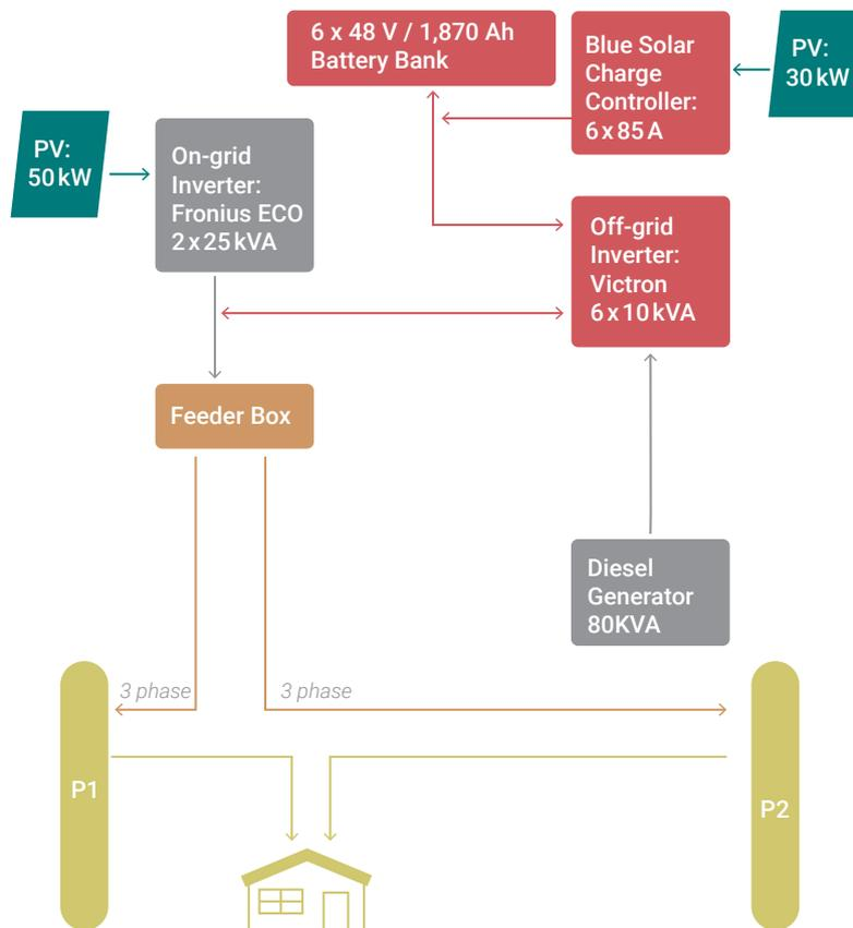
Flooded lead-acid low maintenance Tubular Plate batteries have been considered for the ESS because of its excellent deep discharging capacity, economic viability for such applications, and the expected life under high and extreme temperatures. A diesel-powered generator has been considered for peak shaving or energy deficit from Solar PV modules in bad weather.
