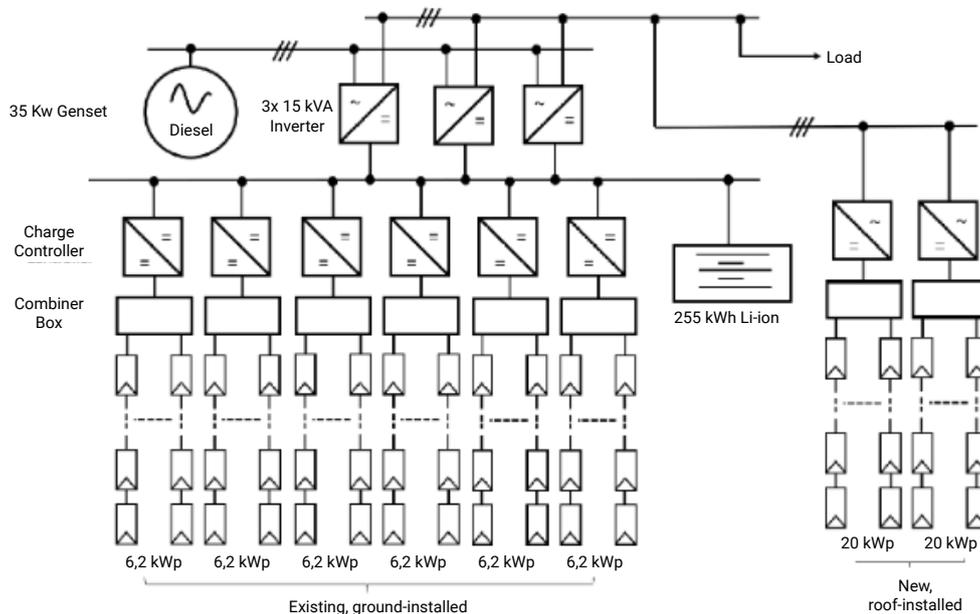
Diagram: PV configurations of 20 kW (ground mount) or 40 kW (roof mount)
