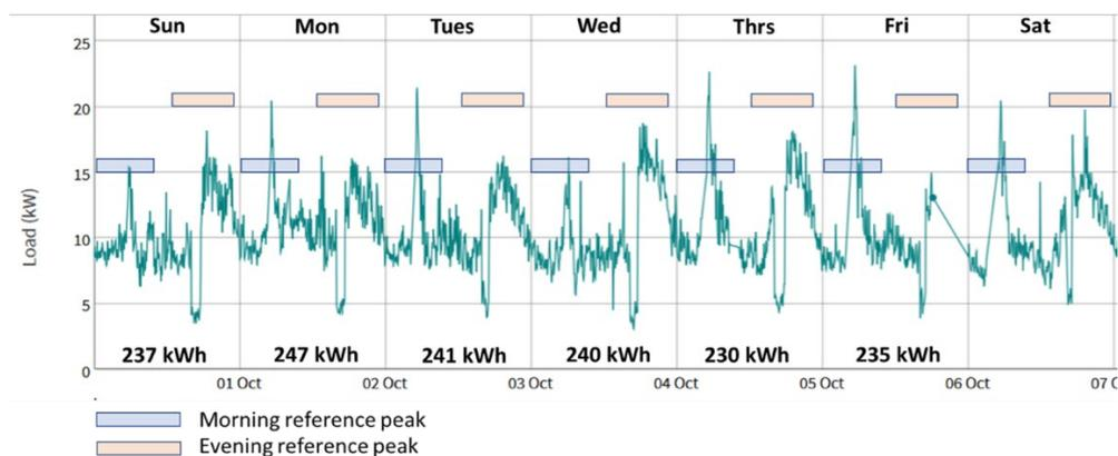
The load profile data shows that the average daily consumption is around 230-250 kWh. The daily consumption reveals clear repetitive patterns with a short morning peak and a longer evening peak. Hence, the daily base load could be directly fed by a new AC-coupled PV array. Based on all data, the project team went ahead and redesigned the system using a holistic approach and software such as HOMER Pro, Helioscope and Excel.
