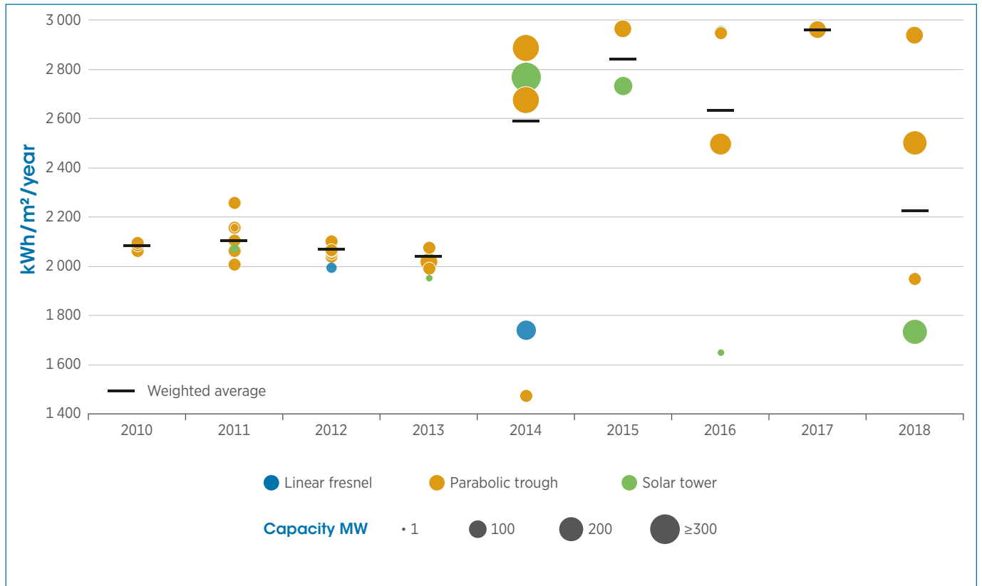
Figure 4.3 Direct normal irradiation levels for CSP projects by year of commissioning and technology, 2010–2018
