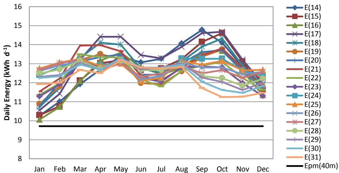
**Figure 44: Energy from  $2.6 \text{ kW}_p$  (optimal inclination angle) and required pumping energy for 40 m borehole category in Mozambique**
