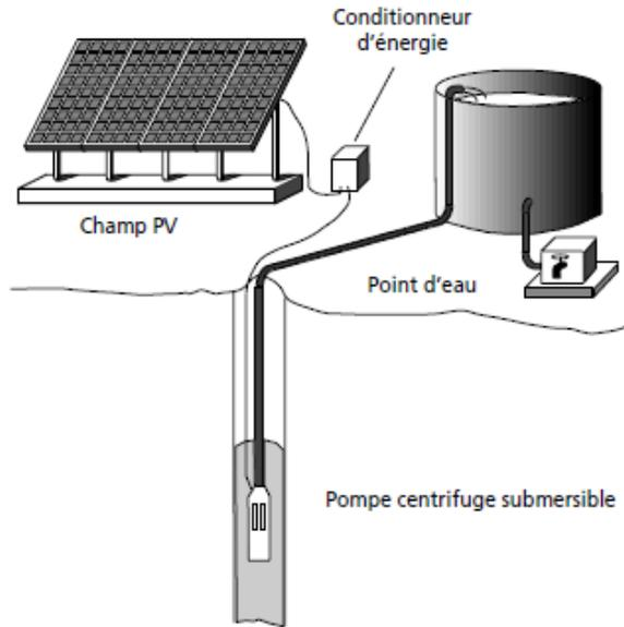
**Figure 20: PV water pumping system (Royer, et al., 1998)**
