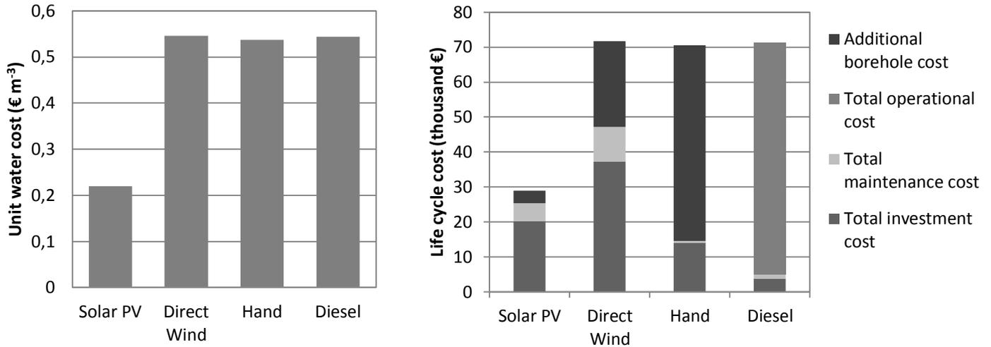
Figure 61: Unit water cost and life cycle cost of the different systems for the 70 m borehole class
