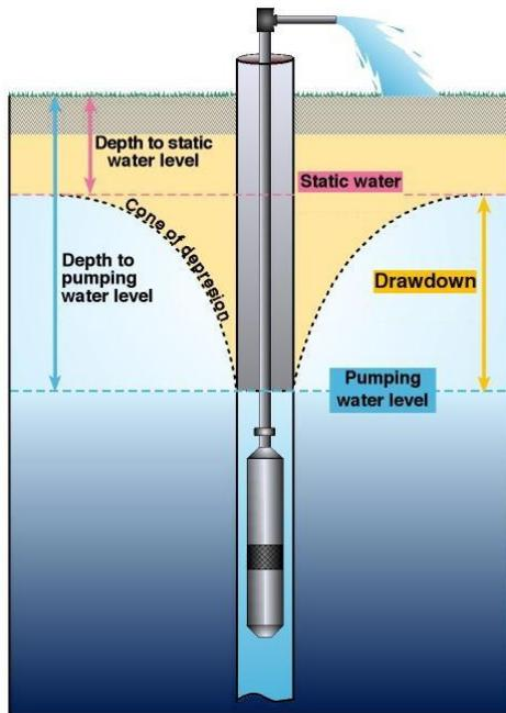
**Figure 15: Water pumping diagram showing the static water level, the pumping water level and the drawdown (Ohio Department of Natural Resources, 2011)**
