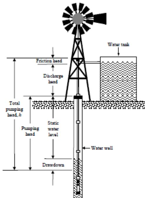
**Figure 25: Windmill pumping system (Argaw, et al., 2003)**
