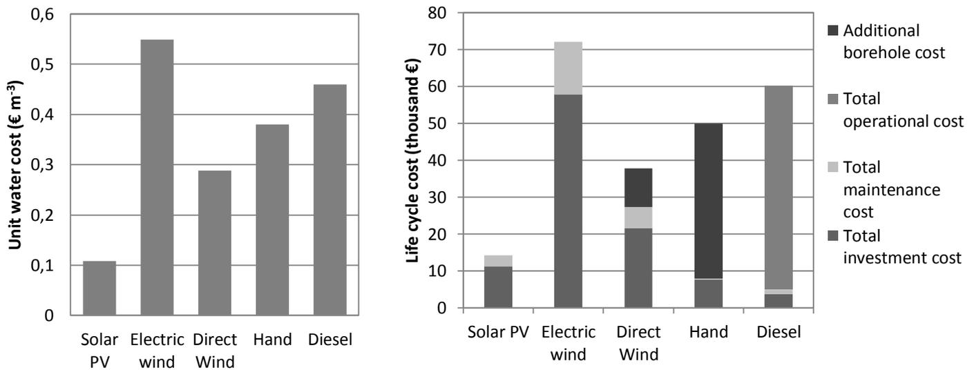
**Figure 60: Unit water cost and life cycle cost of the different systems for the 40 m borehole class**
