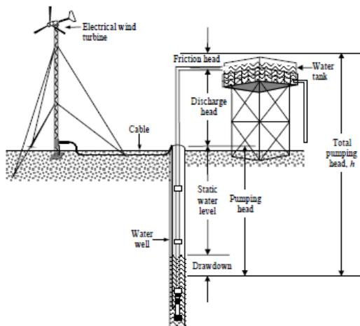
Figure 28: Electrical wind pumping system (Argaw, et al., 2003)
