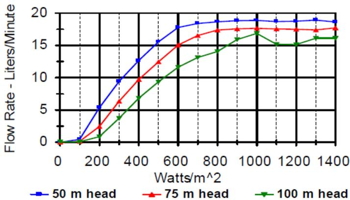
Figure 22: Measured flow rate from a 6 SQF-2 Grundfos pump powered by a 640 W photovoltaic array (Clark & Vick, 2008)
