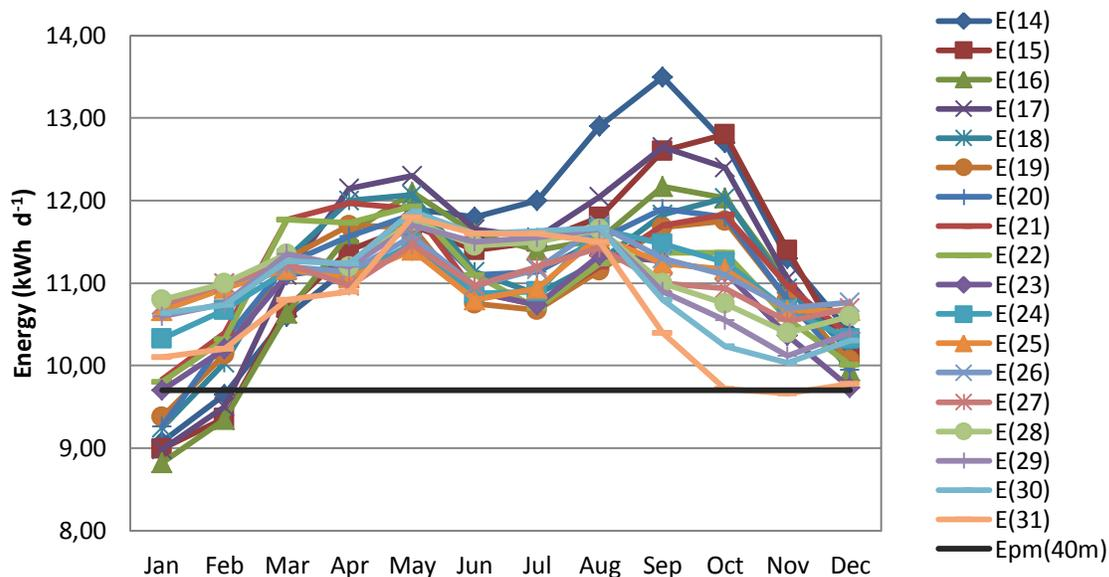
**Figure 46: Electricity production ( $\text{kWh d}^{-1}$ ) from  $2.6 \text{ kW}_p$  for a grid connected system (optimal inclination angle) and required pumping energy for 40 m borehole category in Mozambique (PVGIS European Communities, 2001 - 2007)**
