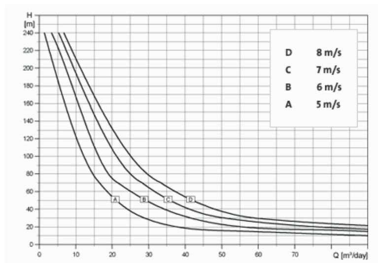
**Figure 30: SQFlex wind performance curve (Grundfos, 2012)**
