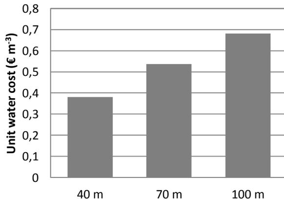
**Figure 58: Unit water cost for the hand water pumping system for the different borehole categories**
