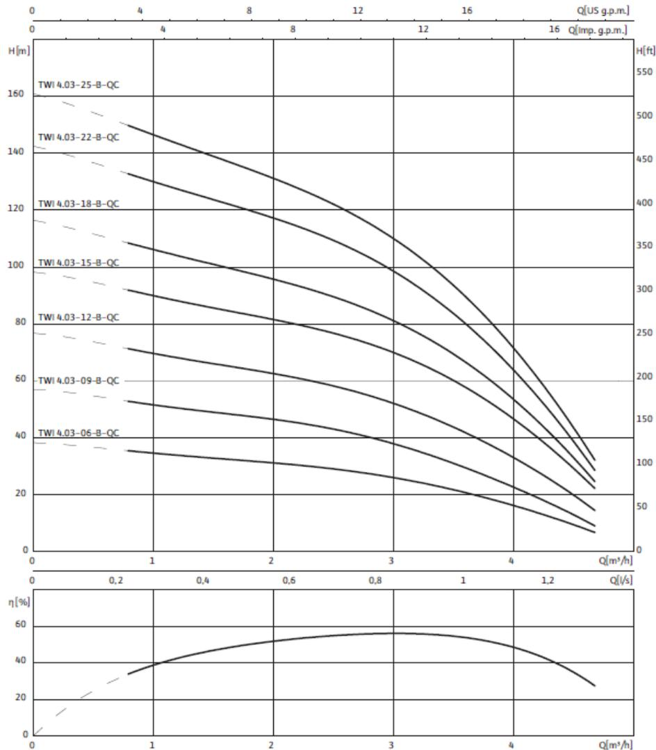
**Figure 8: Pump performance curves for the Wilo-Sub TWI 4.03-...-B-QC types (WILO SE, 2013)**
