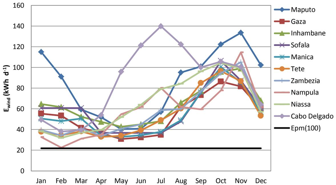
Figure 9: Daily energy from 65 wind turbines (D=2m,  $\eta=30\%$ ) based on mean daily RETScreen wind speed data for every province in Mozambique and pump-motor energy requirement for the 100 m borehole category
