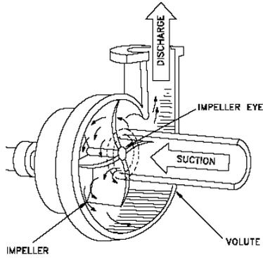
Figure 13: Schematic drawing of a centrifugal pump (Engineers Edge, 2000)
