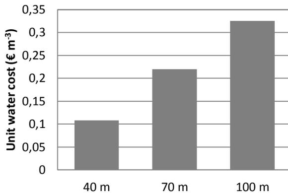
**Figure 56: Unit water cost for the solar PV water pumping systems for the different borehole categories**
