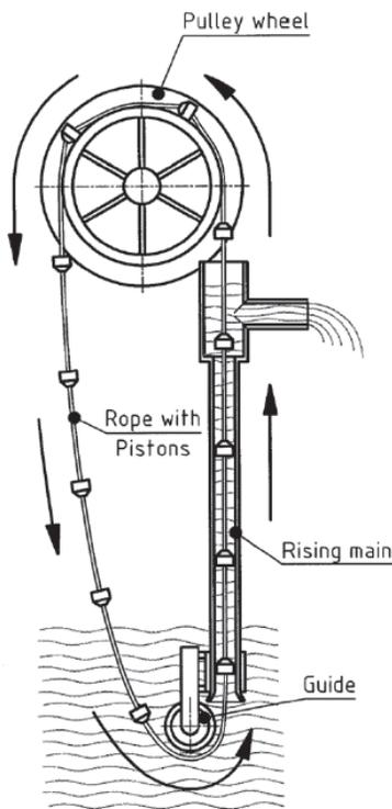
**Figure 9: Scheme of a rope pump (Baumann, et al., 2010)**
