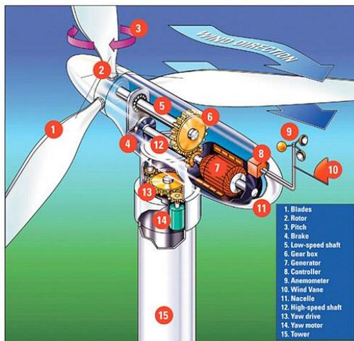
Figure 29: Elements of an electric wind turbine (Alternative Energy News, n.d.)
