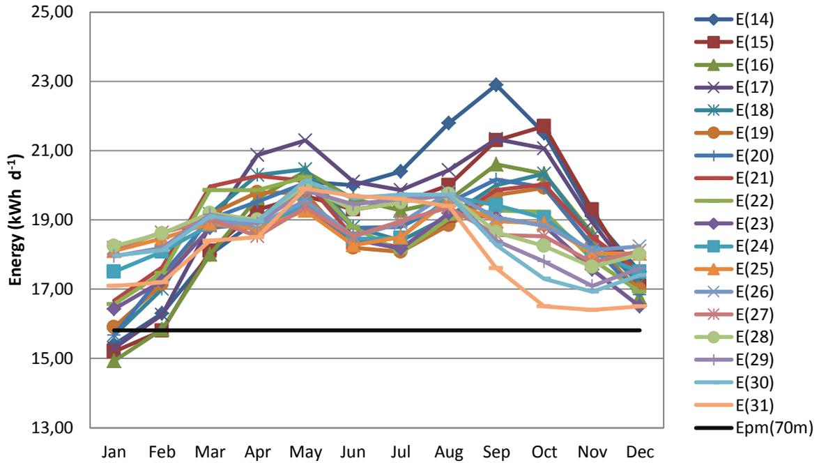
Figure 6: Daily energy production from 4.4 kW<sub>p</sub> optimally inclined grid-connected PV installation for different locations in Mozambique and the pump-motor energy requirement for the 70 m borehole category
