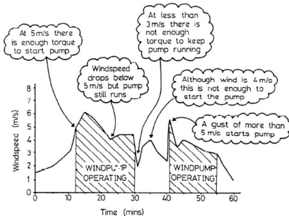
**Figure 27: Illustration of the high wind speed (high starting torque) needed to start the pumping system (Lancashire, et al., 1987)**
