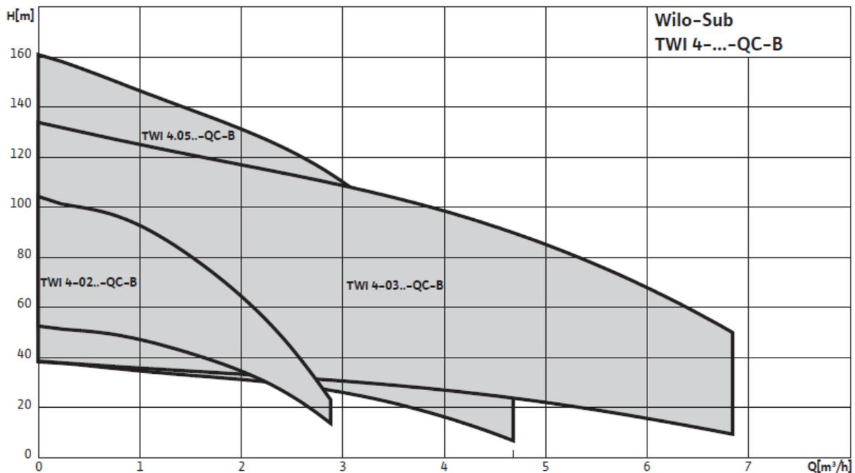
Figure 7: Pumping curve of Wilo-Sub TWI 4-...-QC-B (WILO SE, 2013)
