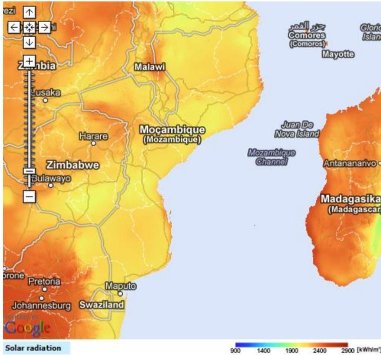
Figure 38: Solar irradiation on a plane with an optimal inclination angle for Mozambique in kWh m<sup>-2</sup> (PVGIS European Communities, 2001 - 2007)
