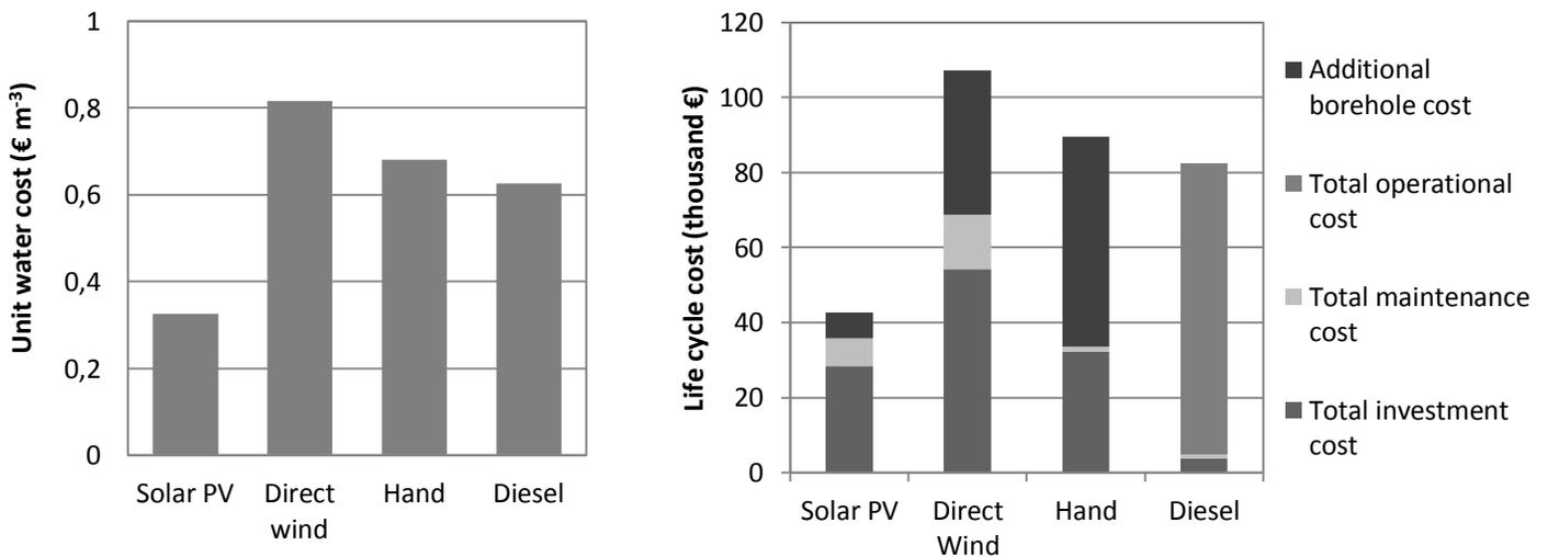
Figure 62: Unit water cost and life cycle cost of the different systems for the 100 m borehole class
