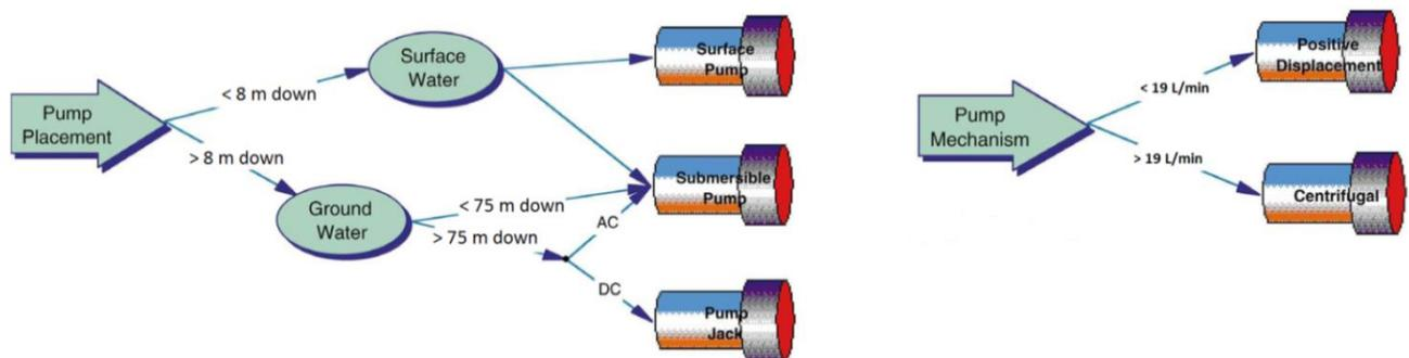
Figure 14: Decision tree for pump type based on (left) placement and (right) demand (Dankoff, 1995)
