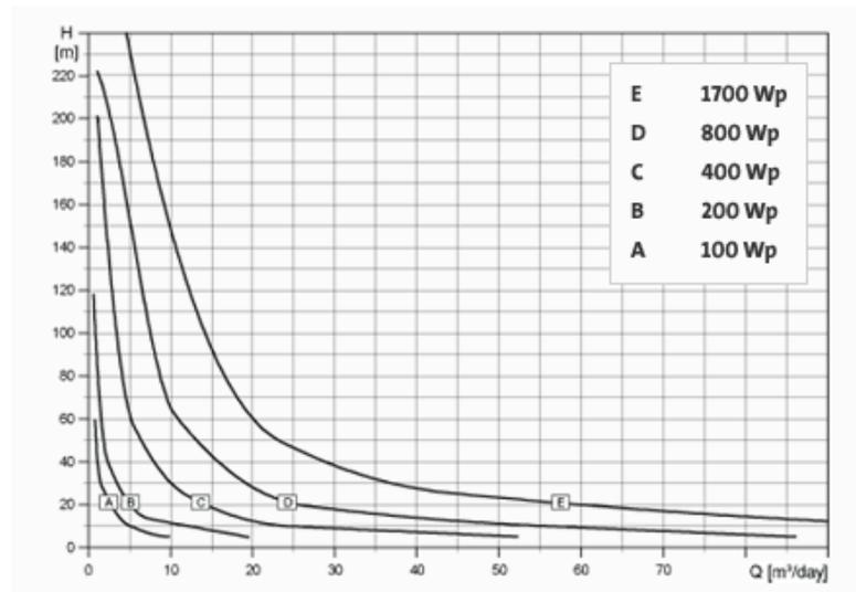
Figure 21: SQFlex solar performance curve (Grundfos, 2012)
