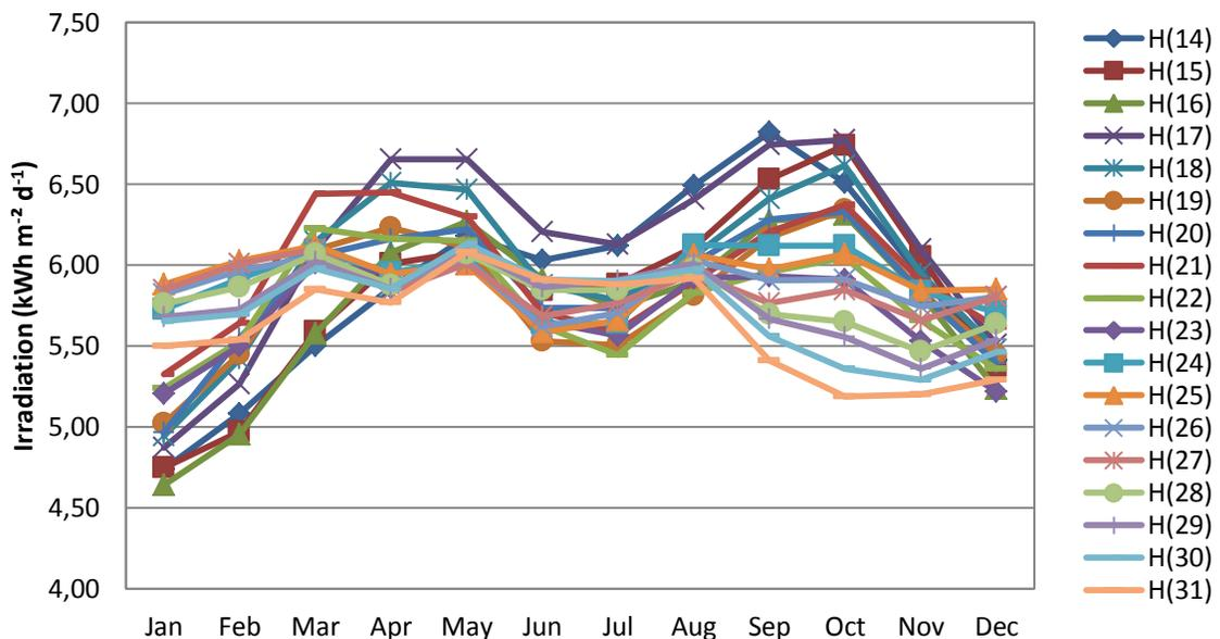
Figure 39: PV GIS data of solar irradiation H (kWh m<sup>-2</sup> d<sup>-1</sup>) on a plane with an optimal inclination angle (given between brackets) in Mozambique (PVGIS European Communities, 2001 - 2007)
