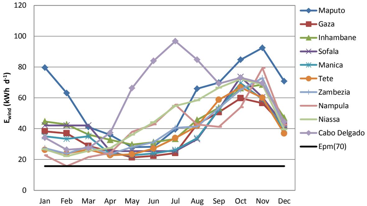
Figure 8: Daily energy from 45 wind turbines (D=2m,  $\eta=30\%$ ) based on mean daily RETScreen wind speed data for every province in Mozambique and pump-motor energy requirement for the 70 m borehole category
