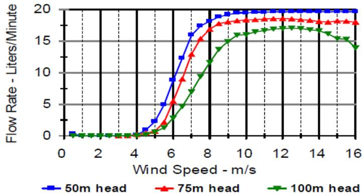
Figure 31: Measured flow rate from a 6 SQF-2 Grundfos pump powered by a 1 kW wind turbine (Clark & Vick, 2008)
