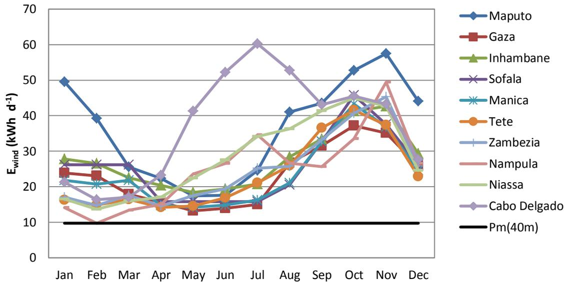
**Figure 51: Energy (kWh d<sup>-1</sup>) delivered by 28 wind turbines for the 40 m borehole category and the required pumping energy**
