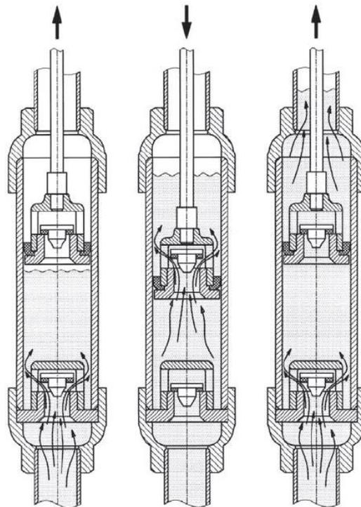
Figure 11: Principle of a reciprocating hand pump (Baumann, et al., 2010)
