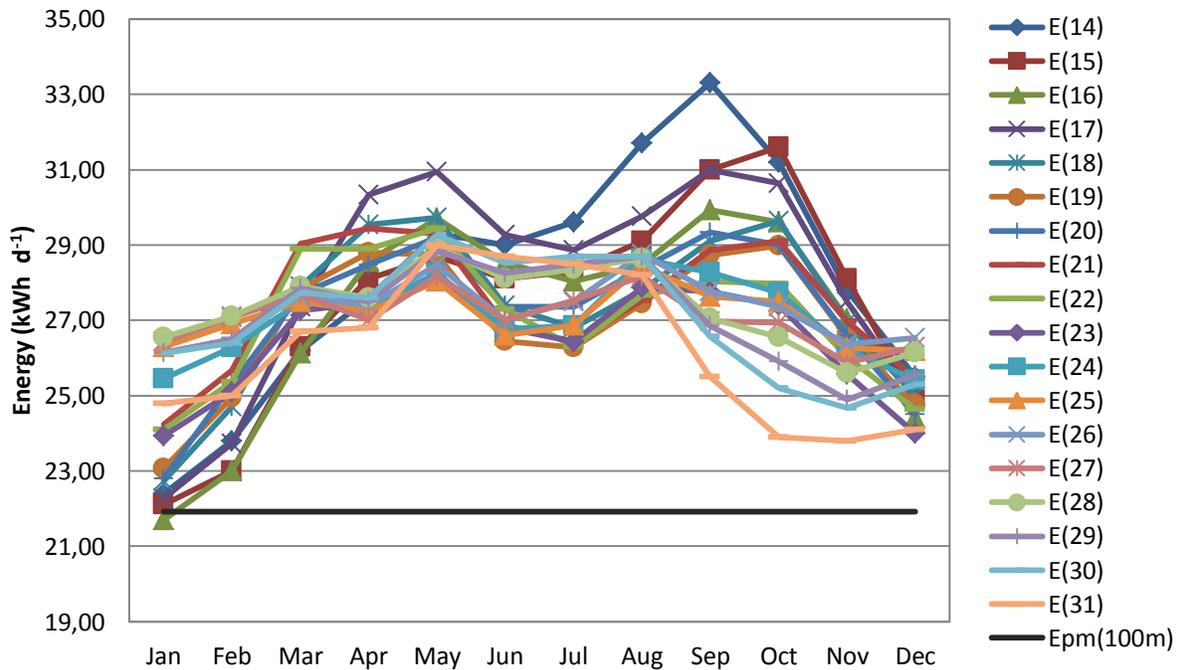
Figure 7: Daily energy production from 6.4 kW<sub>p</sub> optimally inclined grid-connected PV installation for different locations in Mozambique and the pump-motor energy requirement for the 100 m borehole category
