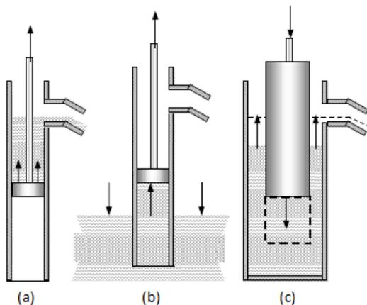
**Figure 12: Basic operating principles of positive displacement pumps: (a) direct lift (b) suction (c) displacement (Argaw, et al., 2003)**
