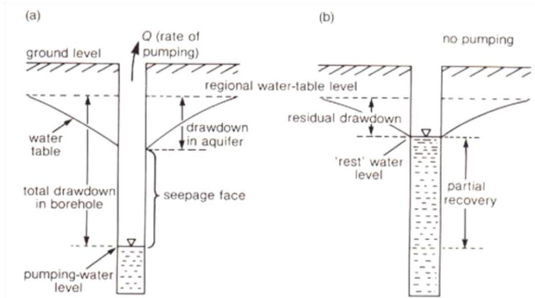
**Figure 16: Water pumping diagram when (a) the pump is running and (b) the pump is not running (Purdue University, 2010)**
