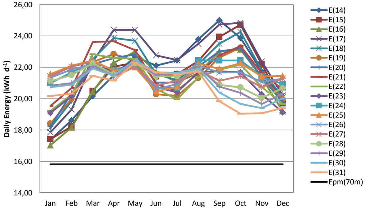
Figure 4: Daily energy from 4.4 kW<sub>p</sub> optimally inclined PV installation for different locations in Mozambique and the pump-motor energy requirement for the 70 m borehole category
