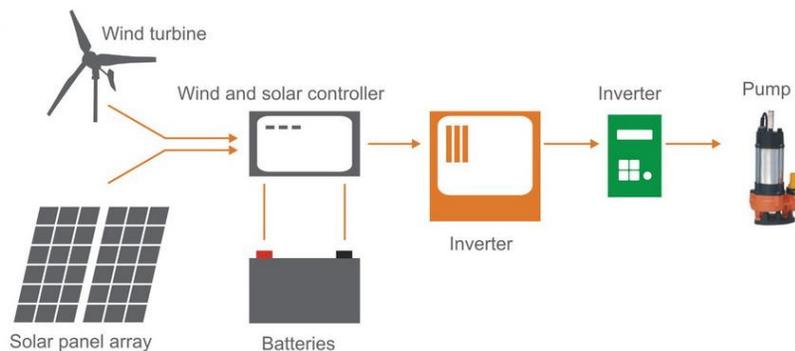
Figure 32: Hybrid water pumping system (Focus Technology Co., Ltd., 2012)
