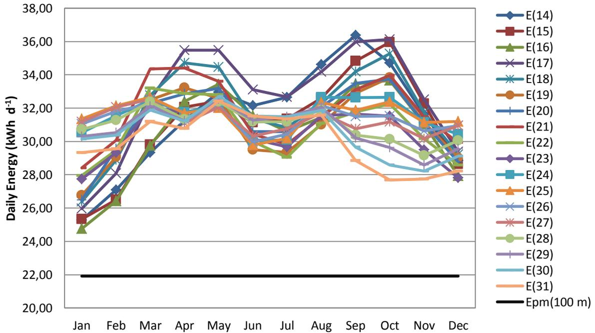
Figure 5: Daily energy from 6.4 kW<sub>p</sub> optimally inclined PV installation for different locations in Mozambique and the pump-motor energy requirement for the 100 m borehole category
