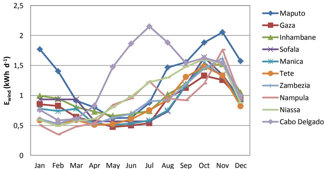
**Figure 50: Daily energy delivered by a wind turbine with a rotor diameter of 2 m per province in Mozambique**
