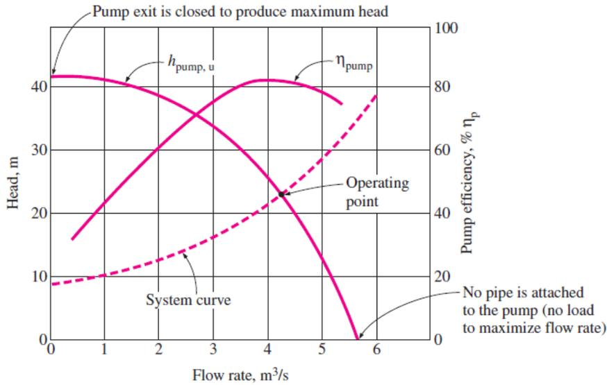
Figure 6: Characteristic pump curve and system curve for a piping system (Cengel, et al., 2008)
