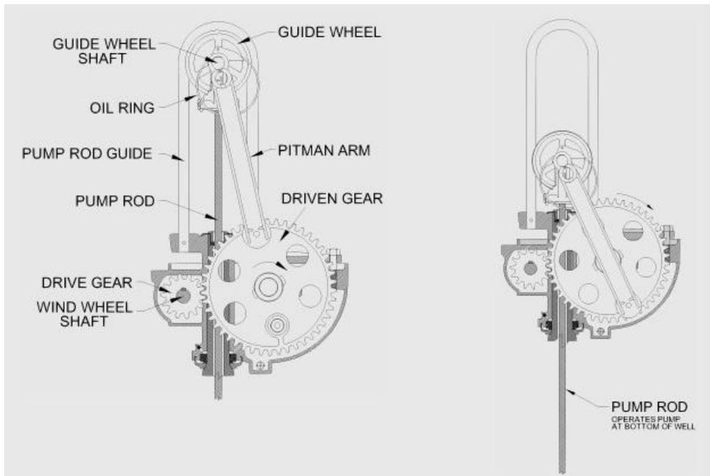
**Figure 26: Working principle of a mechanical windmill (Ironman Windmill, 1970 - 2013)**
