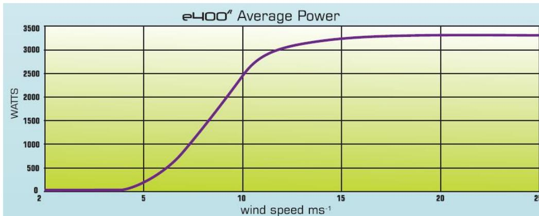
Figure 24: Wind power curve of the e400" Kestrel turbine (Kestrel Renewable Energy, 2012)
