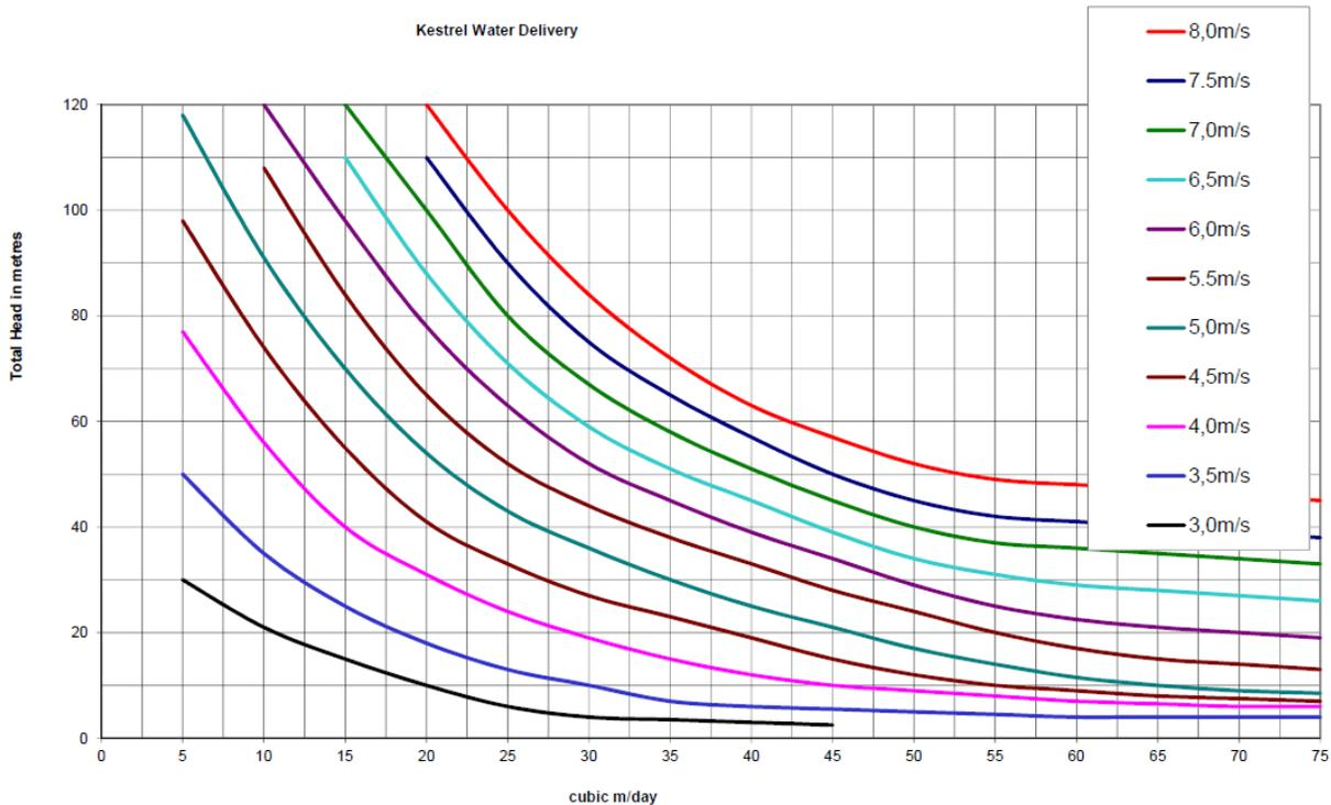
**Figure 52: Water delivery ( $\text{m}^3 \text{d}^{-1}$ ) of e300i (1kW) Kestrel wind turbine for different wind speeds (Kestrel Renewable Energy, 2012)**
