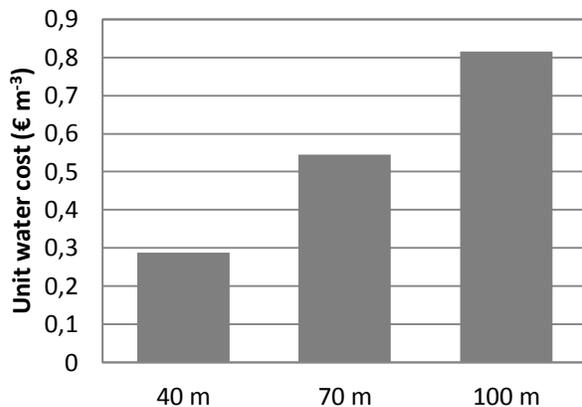
**Figure 57: Unit water cost for the direct wind water pumping system for the different borehole classes**
